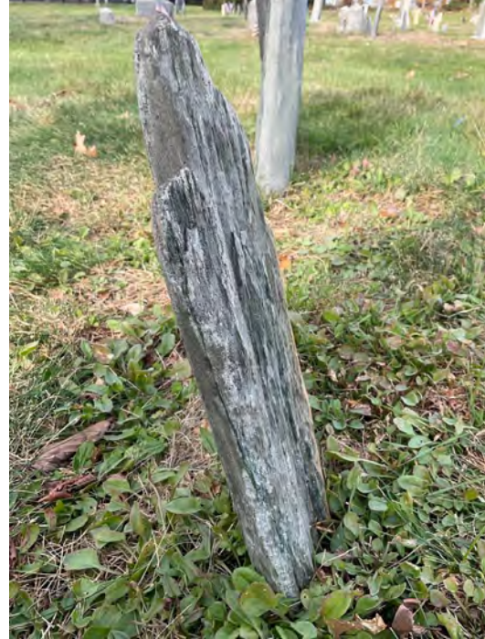
An example of Priority 3 Delamination – the grave marker has only a couple small areas that are treatable; it also has little potential for loss of material of its front face which no longer contains an inscription.
