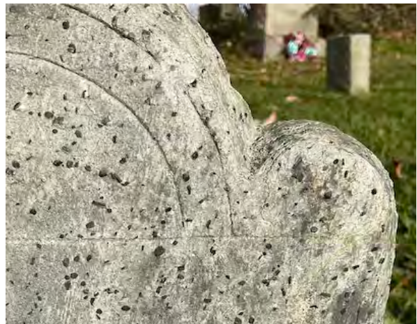
Markers 202 (left) and marker 289_fs (right) are two different slate varieties with prominent iron-rich mineral inclusions.
