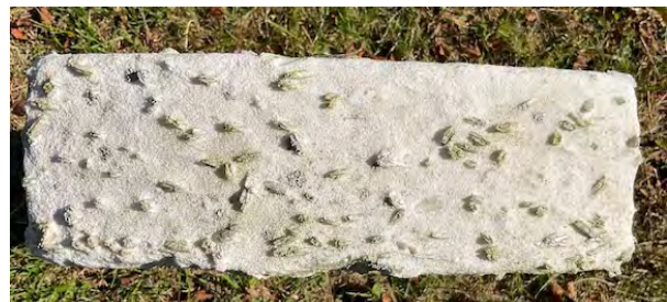
Marker 148 exhibits Disaggregation Severity 4, with fine crystals lost, larger crystals are exposed on the surface. That so much fine particulate has been lost but the surface is not sugaring at present may indicate a consolidation treatment was applied in the past.
