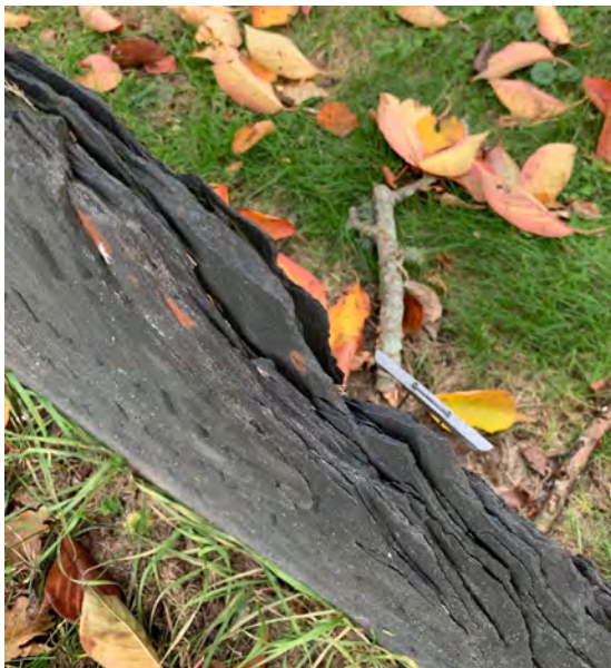
Examples of Priority I Delamination. The bottom right image depicts a grave marker that does not have a number of voids to fill and largely the top delamination is densely packed however there is a small area of delamination on the front that threatens the inscription and is wide enough to receive a fill. This could also be a candidate for a cap due to the intact nature of the top of the grave marker.
