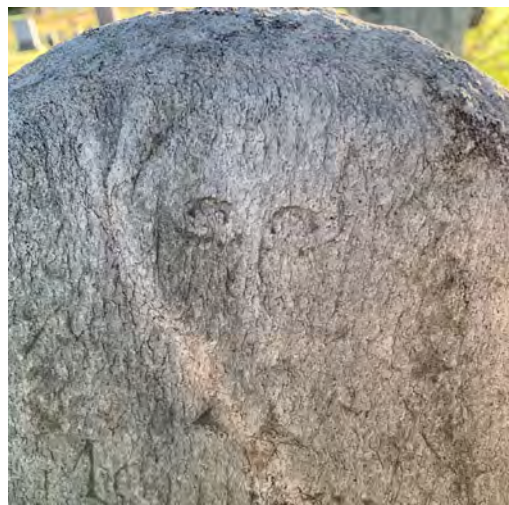
Another example of flaking but it is less densely stacked so presents more potential for loss; also designated Severity I
