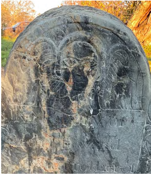
Markers 411 (left) and 290_fs (right) have delamination occurring at the interface of an iron-rich bedding later.
