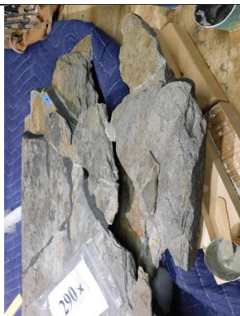
GLA 290x 18. DT. Adhering sections with Akemi Akepox 2030.
