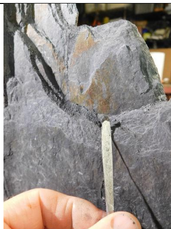
GLA 290x 19. DT. Filling mend-lines and caps with Edison Coatings Systems 45.
