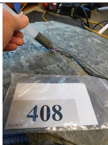
GLA 408 11. DT. Filling openings at mends with Akemi Akepox 2030.
