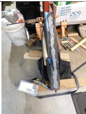
GLA 409 14. DT. Bonding cast with Akemi Akepox 2030.
