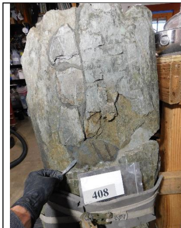
GLA 408 13. DT. Fills and caps with Edison Coatings Systems 45, slate dusts and Bayferrox pigments.
