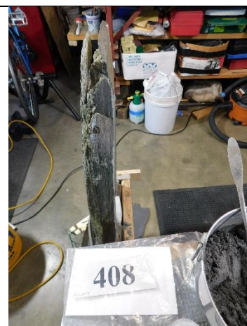
GLA 408 12. DT. Edison Coatings Systems 45 mixed for fills and caps.
