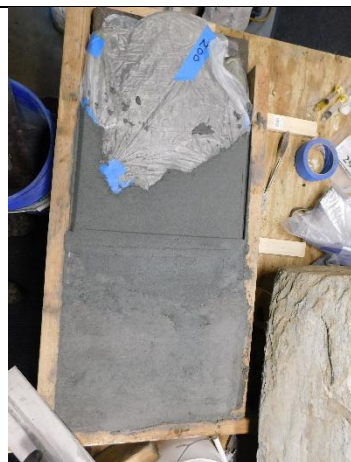
GLA 200 6. DT. Casting missing section with Edison Coatings Systems 45 and Marine Latex.
